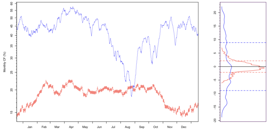
Figure 3: 2023 solar (red) and wind (blue) 30-day MA capacity factors across 2023 at 38°N, 99°W. Subplot at right shows corresponding probability distribution plots of the monthly variability for each resource ( \Delta R_{30d} ). Dotted lines indicate mean \pm 1\sigma .
