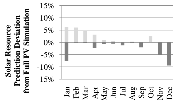
Fig. 10: Monthly energy prediction variation (%) vs. full simulation results for current month, San Jose, CA.
